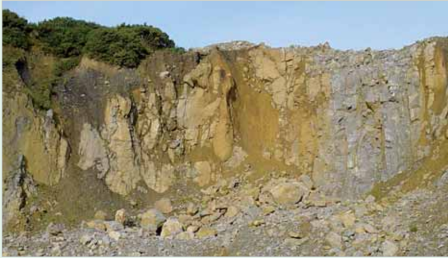
Figure 2-6: Heavily karstified limestone face exposed in a quarry in eastern Ireland. Note the variable depth of dark brown glacial till overlying rock on left hand side of the photograph. Note also the sub-vertical and sub-horizontal nature of discontinuity enlargement and infilling. Karst features are often infilled with soil of Tertiary age (>1.8 million years old). The occurrence of such soils is relatively rare in Ireland (most having been eroded by successive ice ages).
