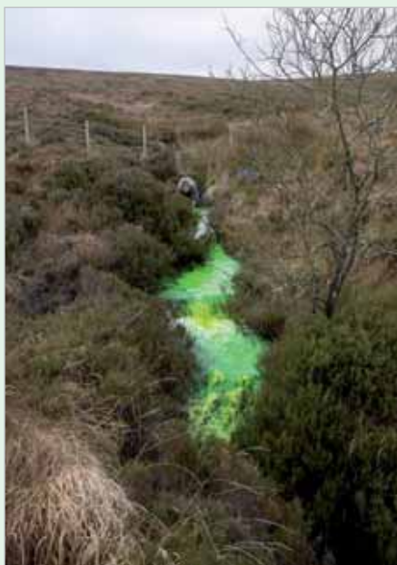
Figure 5-7: Dye-tracing is used to investigate the flow of groundwater in karst aquifers. In this instance, a fluorescent dye is added to upland feeder sinks to establish linkages and flows to springs further downstream.
