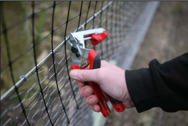
Hog Rings shown in the photo above joining two chain-links together
