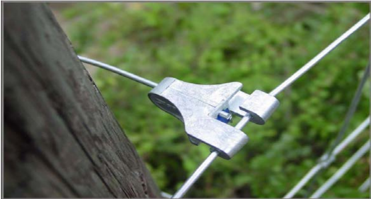
T-Gripple in action as it raps around the strainer posts it returns to grip the horizontal wire
