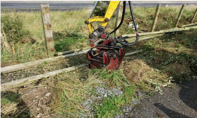
T-Gripple in action as it raps around the strainer posts it returns to grip the horizontal wire
