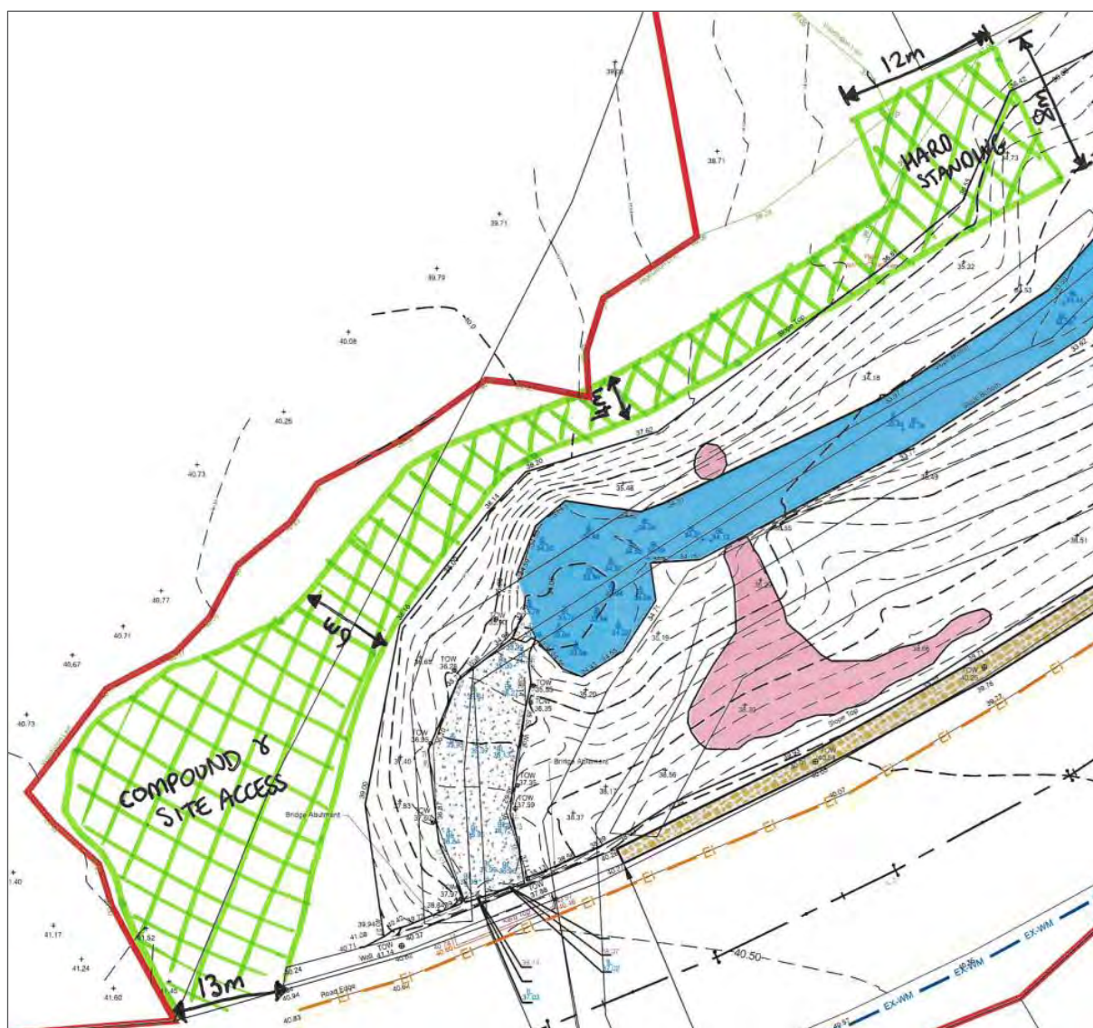
Figure 1-9 - Contractor sketch showing the indicative locations and layouts of the site access and compound areas, access road and hardstanding area north of the stream.
