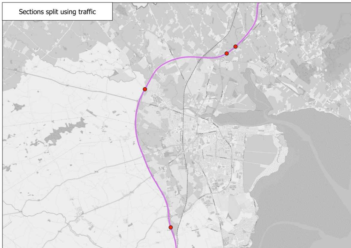
Figure 23: Split into segments around Dundalk by AADT with a threshold of 5000 vehicles per day
