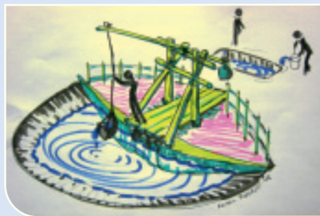
Preliminary reconstruction of the shaduff at Camlin . (Drawing: Niall Roycroft)
