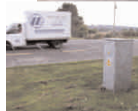
Passing vehicle identified, classified and logged by traffic counter/classifier
