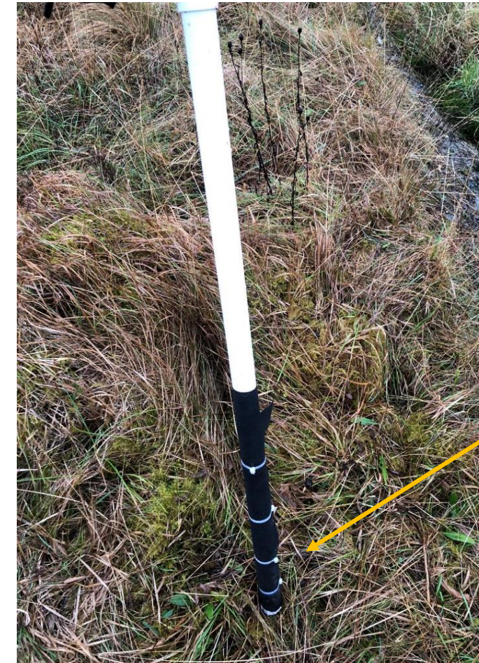
Standpipe with geomembrane prior to installation
