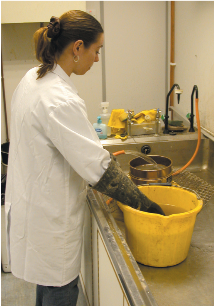
Bulk soil samples are wet sieved to extract plant remains and other inclusions (AOC Archaeology Group)
