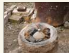
The crucible (containing the ingots) is placed in the furnace and approximately 25–30 kg of high-grade charcoal is used to reach a temperature of 1,500° C. This process takes roughly 30 minutes using a hand-operated bellows.
