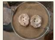
The heated moulds are readied for the casting. The small holes, or risers, to the side are to release gases that form within the empty mould when the bronze is poured.
