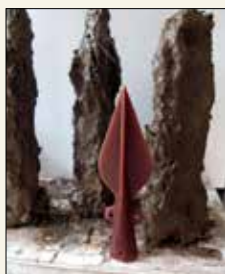
The moulds for the casting are formed around the wax replicas. The moulds are made from river clay, horse manure and sand, which is left to dry for several weeks. This forms a slightly breathable material that can withstand intense heat while releasing the gases produced during the casting.
