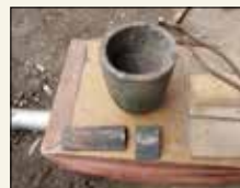
The copper and tin ingots (foreground) are ready for the crucible, where they will be combined to form bronze. Crucibles and their fragments are important indicators of metal-working activity on archaeological excavations.
