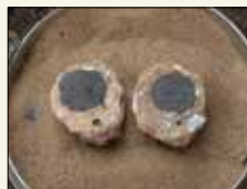
The bronze cooled and set, as seen by the change in its colour. Oxides in the metal are responsible for the black surface colour.
