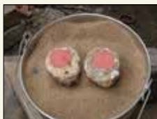
The bronze is allowed to rest in the mould, to fill the entire cavity and to set.
