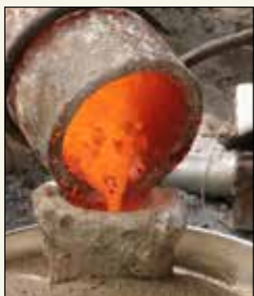
The molten bronze is poured into the mould. This is the most critical time of the casting, when many hours of work are at stake.
